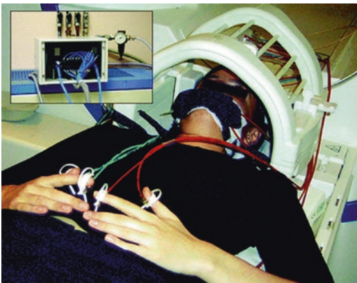
Fig. 18.6 Fully automated pneumatically driven tactile stimulation. Flexible membranes (4D Neuroimaging, Aachen, Germany) connected to pressure-resistant pneumatic tubes transmit the stimuli to the lips, fingers, or toes (not shown). Upper left: the 24-channel high-precision electromagnetic valve system was designed to investigate somatosensory somatotopy (Reprinted from Stippich 2007, p. 94, with permission)
