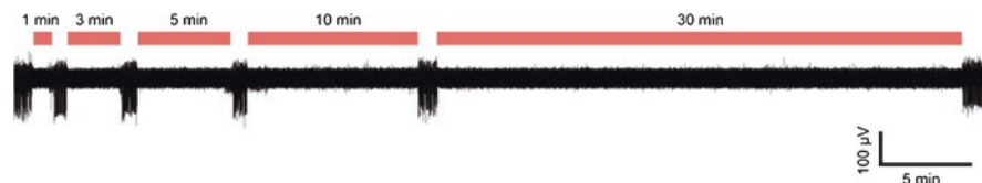
Fig. 14.4 Inhibition of neural activity by photothermal effect of gold nanorods under NIR light. Positively charged gold nanorods were electrostatically attached to neurons' plasma membrane, and a train of neural spikes showed inhibition of neural activity during irradiation and restoration upon the removal of irradiation (Yoo et al. 2014). (The figure was adapted with copyright permission from Yoo et al. (2014), © American Chemical Society 2014)
