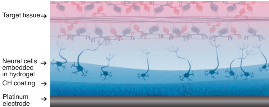
Fig. 7.15 Schematic of layered “living electrode” design. (Reproduced with permission from Goding et al. (2017))
