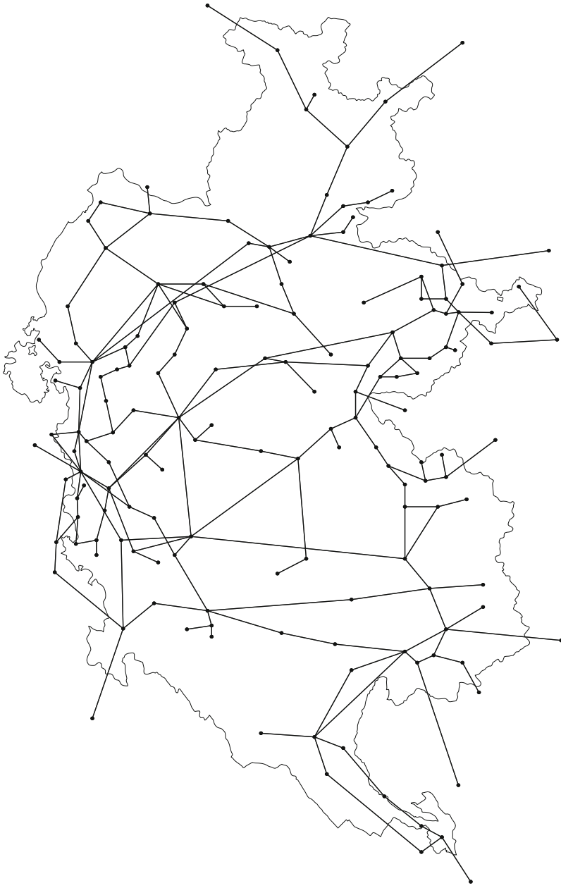
Fig. 2 The Swiss maximum voltage power grid as a graph with 159 nodes and 394 edges (simplified representation)
