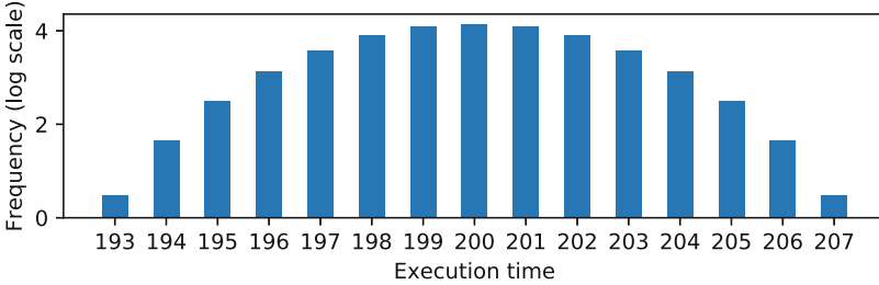
Fig. 1. Frequency of the occurrence (in absolute numbers) of a certain execution time (in cycles) of the __udivmodhi4 function for all 2^{16} possible 16-bit unsigned integers.
