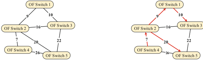
(a) A weighted graph of network traffic (b) The forwarding path in data plane
