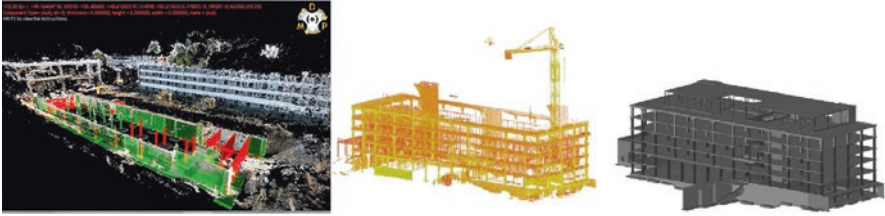
Fig. 5.5 Progress is shown in as-built and 4D BIM models with color-coded status superimposed together (left) (Golparvar-Fard et al. 2012), laser scanned as-built (middle) and 4D BIM model (right) (Turkan et al. 2012)
