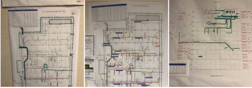
Fig. 5.8 Examples of printed 2D drawings with highlighted progress to communicate the actual status, this process is time-consuming and labor intensive
