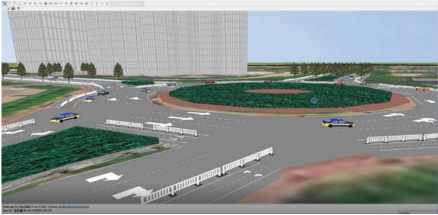
Fig. 14.9 Real-time microscopic traffic simulation: FLOWSIM
