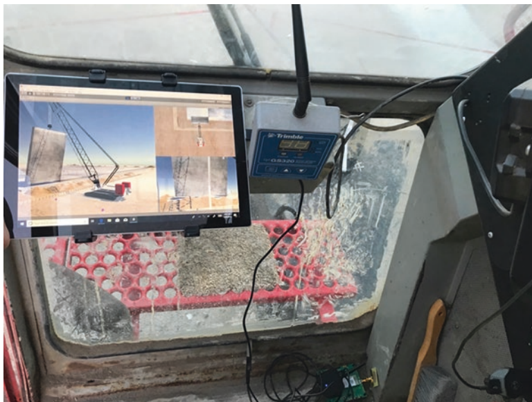
Fig. 11.17 Tablet deployed in the crane cabin for lifting scene visualization and potential hazard identification
