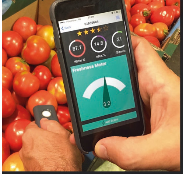
Fig. 12 Using a mobile application for measuring fruits and vegetables ripeness quality, freshness, durability, and taste (Clairfruit, 2018)
