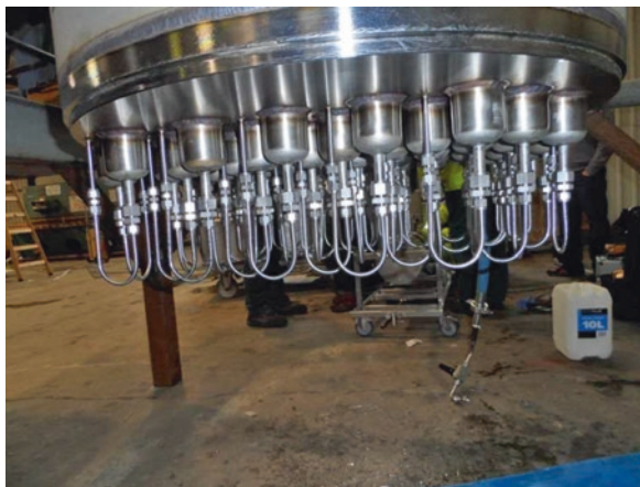
Fig. 2.7 Picture of a bottom of pipes and jumpers for a 360 L vertical pipes-in-series PFR for two-phase reactions with reagent gas used in GMP production
