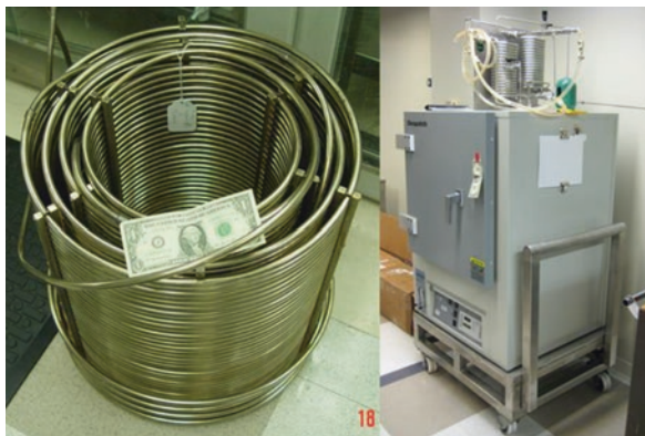
Fig. 2.2 Picture of a 7.1 L coiled tube thermal PFR (left) and forced convection oven for heating the reactor inside (right)
