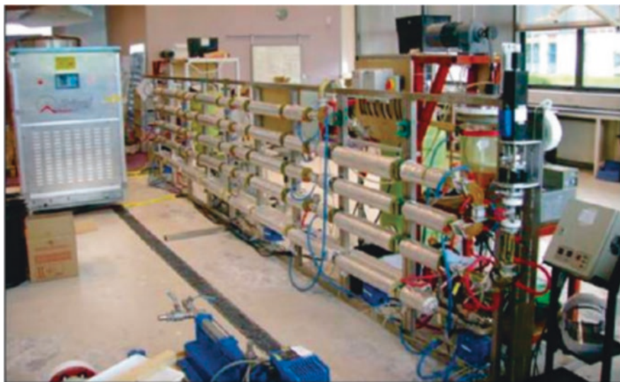
Fig. 5.30 A custom-built stainless steel OFBC unit. (Permission obtained from Lawton et al. Copyright © 2009, American Chemical Society)
