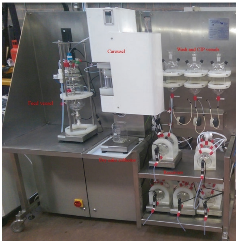
Fig. 5.45 A continuous filtration drying unit developed by AWL. (Permission obtained from Ottoboni et al. © 2019 American Pharmacists Association®. Published by Elsevier Inc.)
