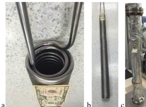
Fig. 2.9 Pictures of 2.5 L Hastelloy coiled tube PFR (a, b), and (c) insulated steam jacket pipe for temperature control
