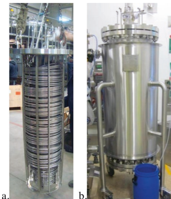
Fig. 2.8 Pictures of (a) 12 L Hastelloy coiled tube PFR, and (b) steam jacket pipe for temperature control
