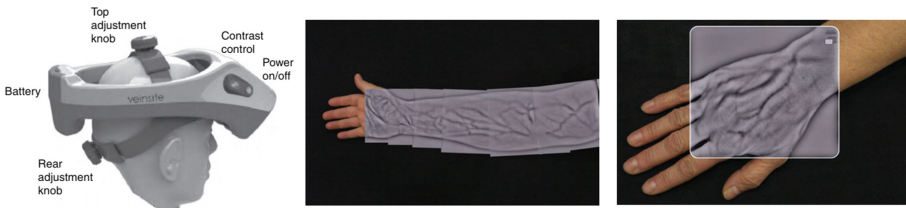
Fig. 2. The Veinsite™ headset diagram (left) and View of upper extremity veins (center and right) (Source: [18], p. 967).
