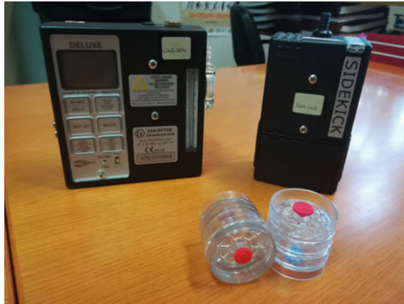
Fig. 1 Suction pumps and cassettes used for sampling
