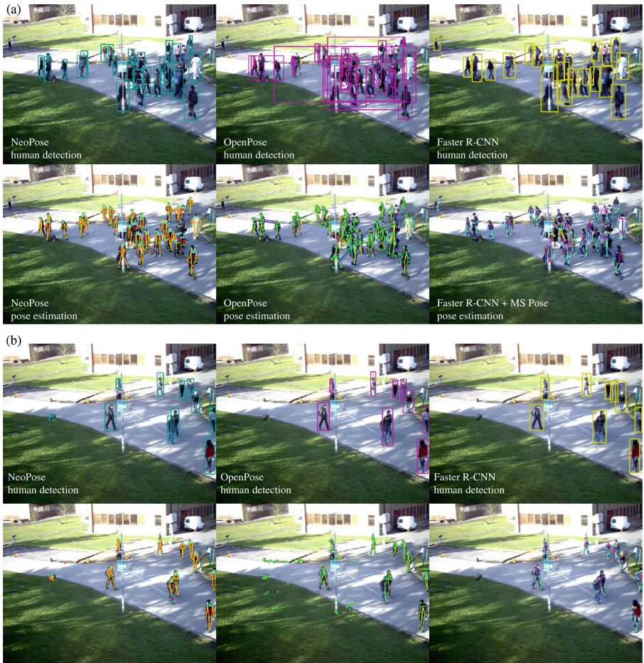
Fig. 10. Comparisons of human detection and pose estimation on surveillance images of a pedestrian crossing (MOT dataset) using different algorithms. (a) and (b) are two representative moments.
