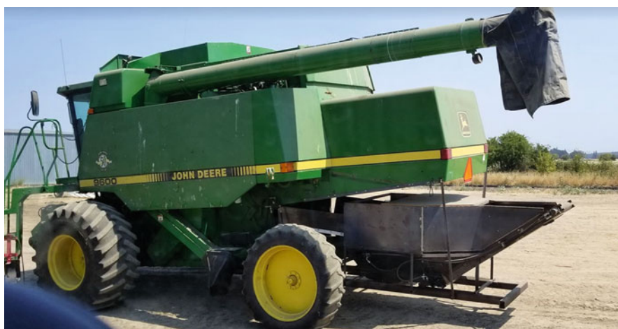
Fig. 3.6 This combine has been modified by placing a bin underneath to collect hemp chaff which comes from around the seed grain and could potentially be suitable for extraction. (Source: John Fike)
