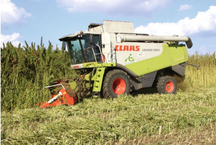
Fig. 2.3 A modern French forage chopper for cutting and windowing hemp. (Source: G. Chanet, Eurochanvre, Arc-les-Gray, France)
