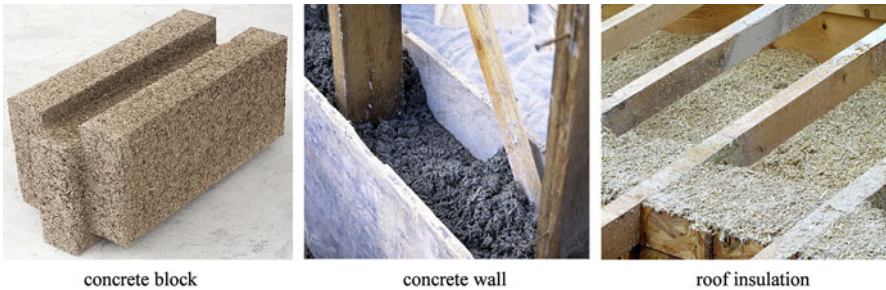
Fig. 2.6 Hemp-based products for insulation or building. (Source: G. Chanet, Eurochanvre, Arc-les-Gray, France)
