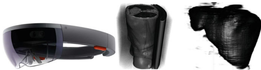
Fig. 1 3D visualization of liver segmentation in Microsoft HoloLens (left): the segmented liver volume (right) was separated from the input volume—a scanned torso (center). Source: authors
