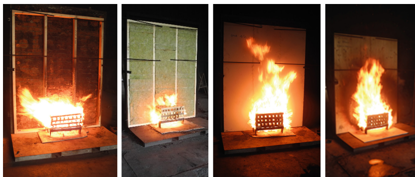
Fig. 1. Samples of 1800 × 2300 mm wood components during fire testing (fire spread).
