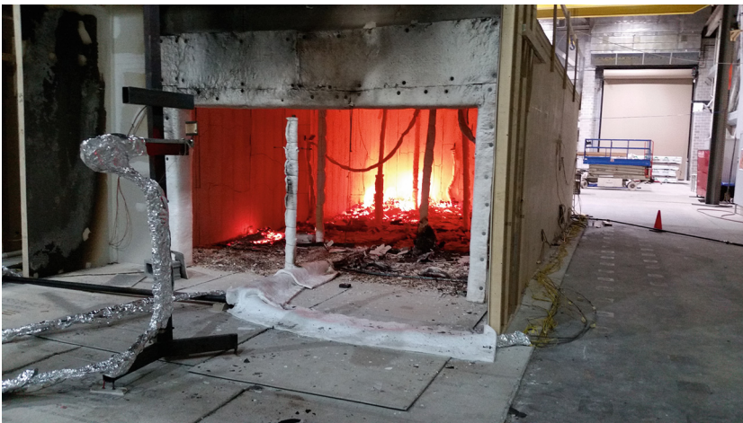
Fig. 1. CLT compartment fire from the Fire Protection Research Foundation series of tests (undertaken by National Research Council, Canada with RISE, Sweden, at the National Institute of Standards and Technology) (image, Arup)
