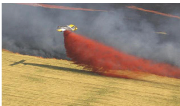
Fig. 1. Single engine aircraft releases long term fire retardant front of a low intensity fire line [14]
