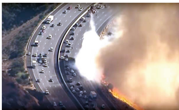
Fig. 2. Helicopter pilot began water release some seconds later than the optimal place requires [15]
