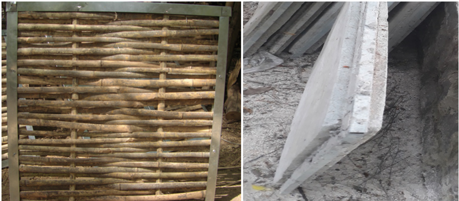
Fig. 1. Inter-woven bamboo strips inside the metallic frame and fully cast panel.
