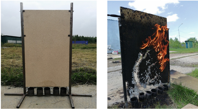
Fig. 3. Photographs of the wood-base panel during field fire tests.
