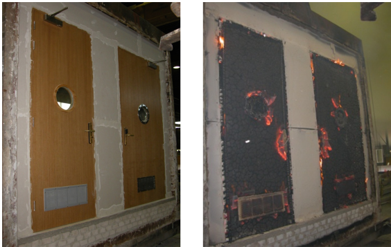
Fig. 2. The view of the exposed side of tested specimen prior (left side) and after (right side) the test
