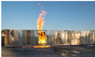
Fig. 1. 30 min propane gas fire engulfment of wood filled impact limiter in the BAM TTS fire test facility.
