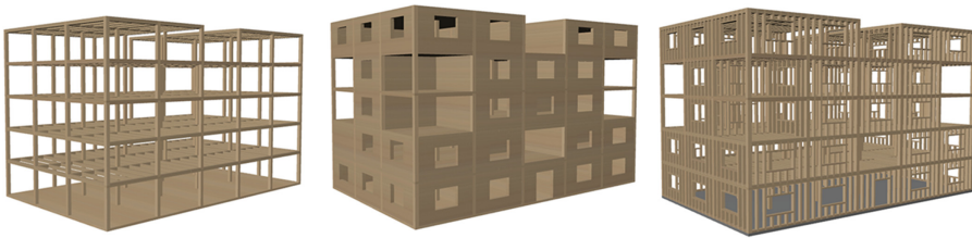
Fig. 1. The load-bearing systems currently used in timber buildings (left to right): timber skeleton; panel system - solid glued-wood structure; non-structural perimeter wall pillar framework combined with skeleton.
