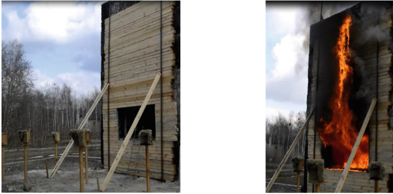
Fig. 1. Photo of a building fragment to simulate fire load and photo of a moment of the experimental study.
