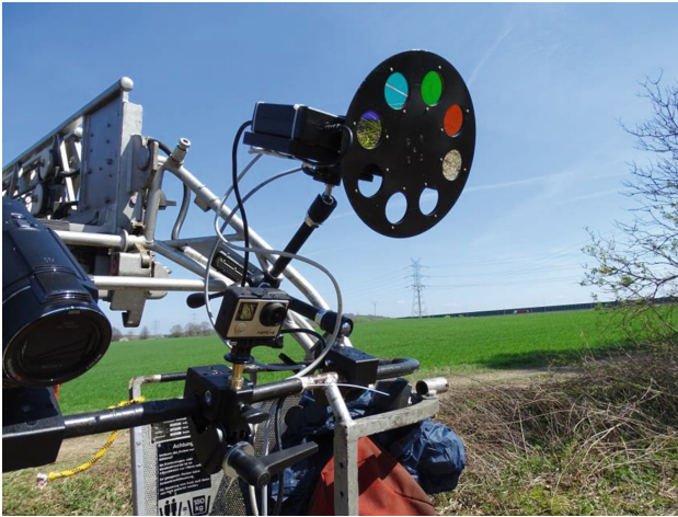
Fig. 1. Monochromatic camera with automatic band-pass filter changer.
