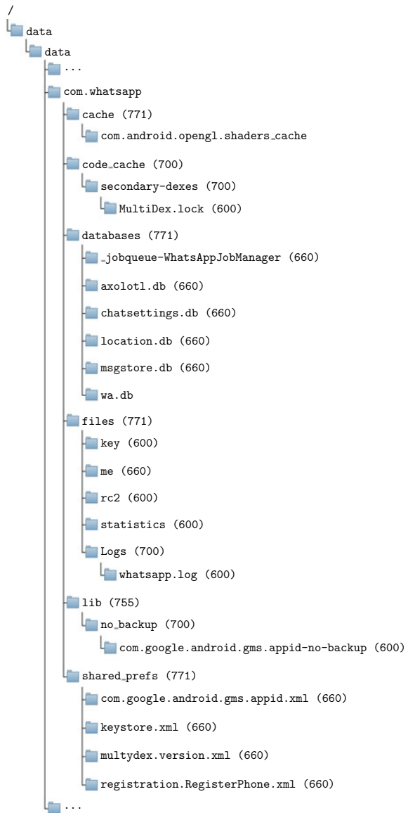
Fig. 13.7 Partial structure and permissions of the folder that Whatsapp is installed as recorded in the rooted phone
