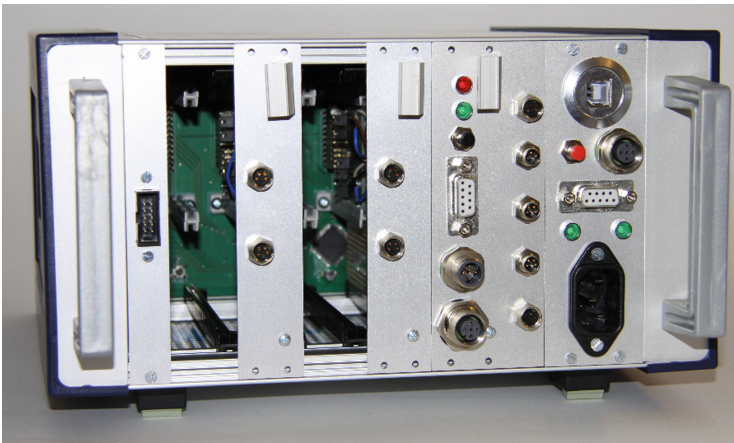
Fig. 5. Aluminum housings used at the distilling apparatuses equipped with two temperature boards, two vacant general connections slots and the power board.
