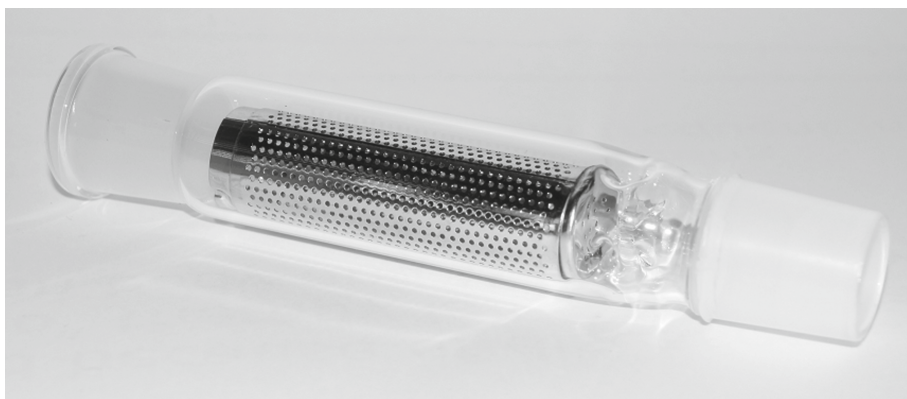
Fig. 3. The smallest size of Hempel column with a stainless steel tea filter for hosting of flavor adding additives
