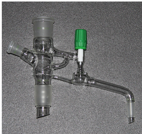
Fig. 2. The reflux separator used for the outflux control of the large setup
