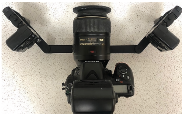
Fig. 6.6 The “3–2” flash position used for most intraoral photos
