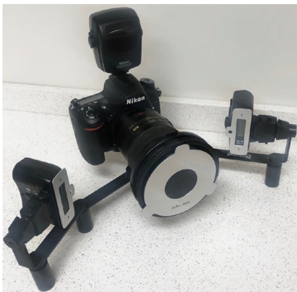
Fig. 6.36 A Nikon dual flash setup with Polar_Eyes affixed to the lens and flashes, in 3–2 flash position
