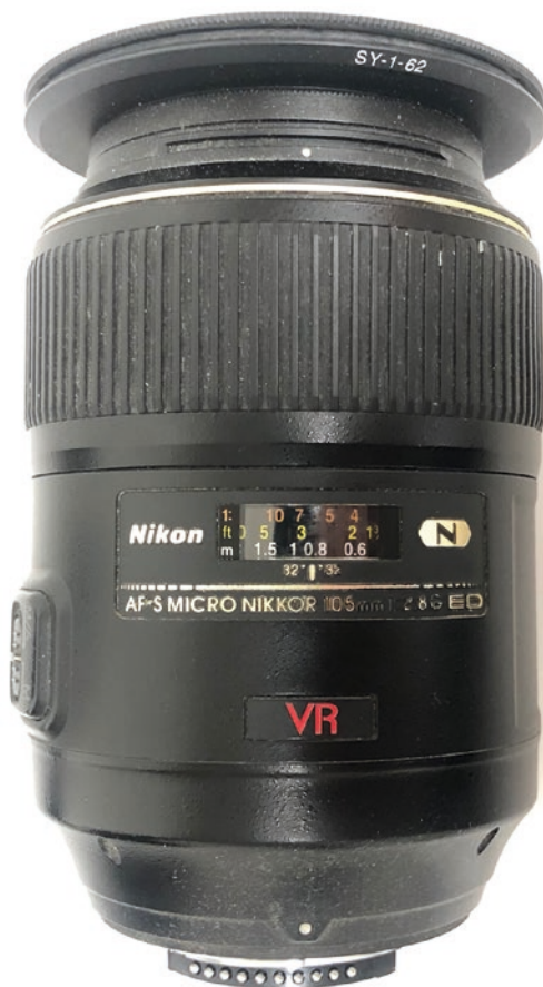
Fig. 6.8 A Nikon 105-mm macro lens, showing the magnification markings
