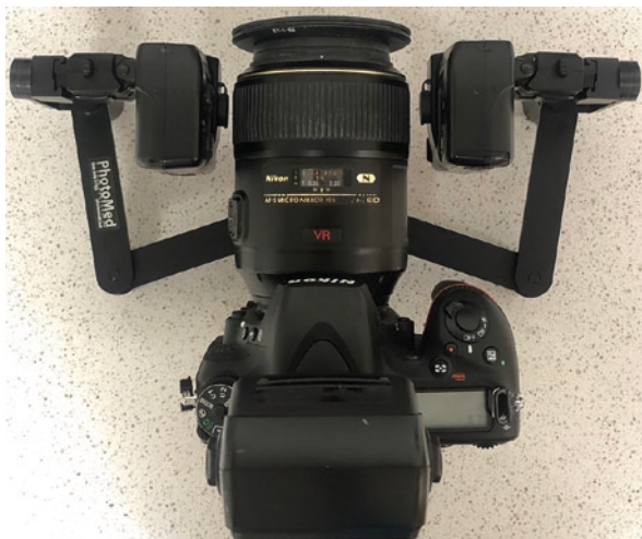
Fig. 6.5 The “next to lens” flash position, used only for occlusal (mirror) shots
