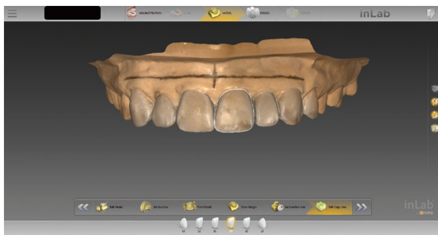
Fig. 11.17 The copy lines (white) are drawn on the wax-up digital impression and matched with the abutment teeth
