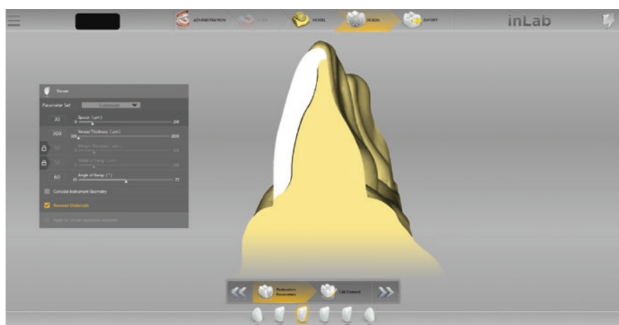
Fig. 11.42 The restoration parameters as the virtual spacer, the veneer and the margin thickness, the interproximal contact strength etc. are set
