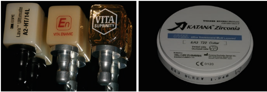
Fig. 8.1 On the left, examples of CAD/CAM block trademarks: base-resin material (Lava Ultimate), polymer-infiltrated ceramic network (Vita Enamic), and zirconia-reinforced lithium silicate (Vita Suprinity). On the right, an example of CAD/CAM disc of ultra-translucent multilayered zirconia (Katana Zirconia)
