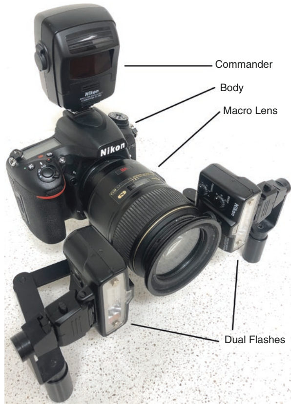
Fig. 6.1 A Nikon D750 setup with a commander, macro lens, and dual flashes mounted on brackets
