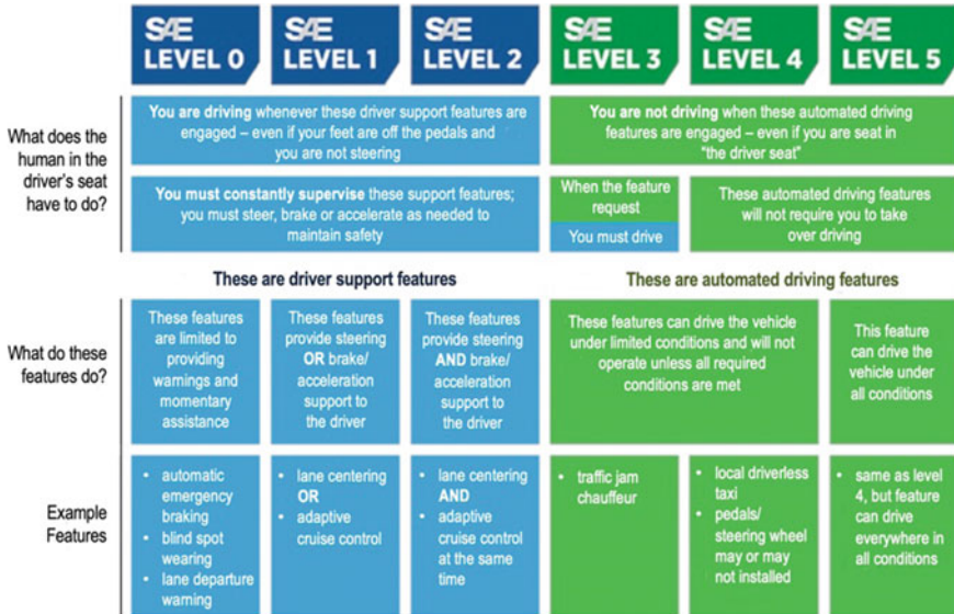
Fig. 12.3 Levels of driving automation by SAE international’s J3016 standard. ( https://www.sae.org/ )
