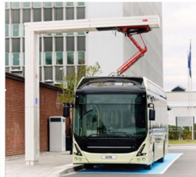
Fig. 11.3 Different modes to recharge the electric buses. a Plug-in charging and b pantograph charging (ABB 2019)
