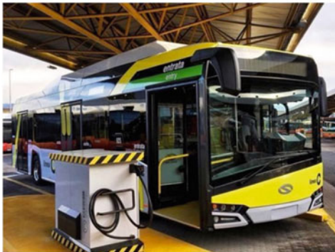
Fig. 11.3 Different modes to recharge the electric buses. a Plug-in charging and b pantograph charging (ABB 2019)
