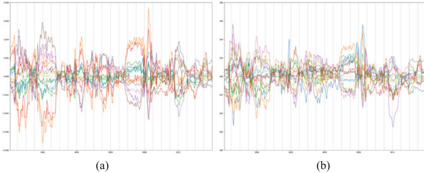
Fig. 8.11 The reconstruction error in Y is shown for (a) the linear encoder and (b) a deep autoencoder, with two \tanh activated layers for each of the encoder and decoders
