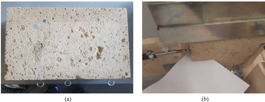
Fig. 8. Testing surface: (a) roughness of tested surface and (b) contact surface of the tested specimen
