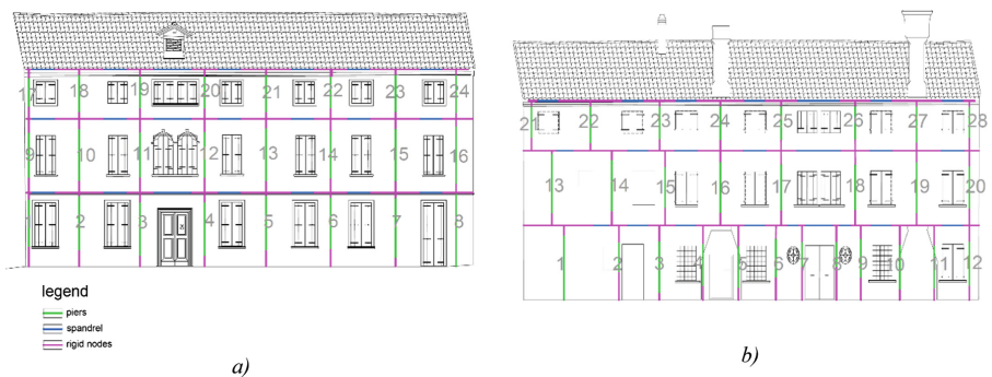
Fig. 5. (a) EFM of main elevation (frame-like); (b) EFM of rear elevation (non-frame-like).
