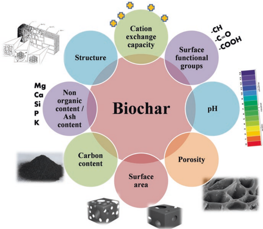
Fig. 4.2 Characteristic physico-chemical properties of biochar
