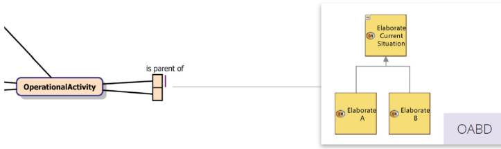
Fig. 3. An ORM-fact type expressing that an “Operational Activity” can be a parent of another “Operational Activity”
