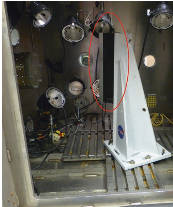
Fig. 10.12 Impact testing fixture secured in impact chamber
