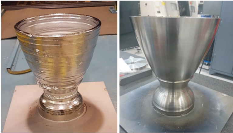
Fig. 8.9 Generic Ti-6Al-4V rocket nozzle as-built (left) and after machining (right). (Image credit: NASA)
