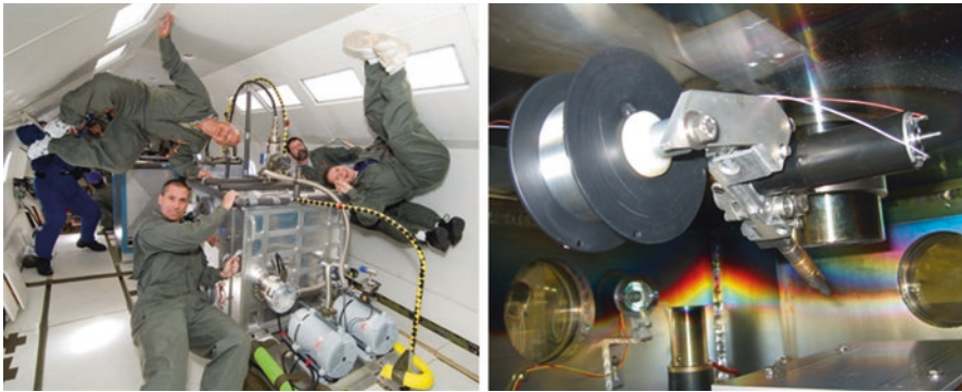
Fig. 8.4 First-generation portable, fixed-gun EBF 3 system undergoing 0-g testing in parabolic flights. (Image credit: NASA)
