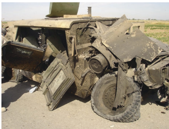
Fig. 1.1 Remains of an armored Humvee military vehicle after being struck on the right side by single man-driven, forward-loaded suicide vehicle-borne improvised explosive device, Iraq, 2005. (Photo: Staff Sgt. John B. Francis, USMC. Courtesy US Department of Defense)
