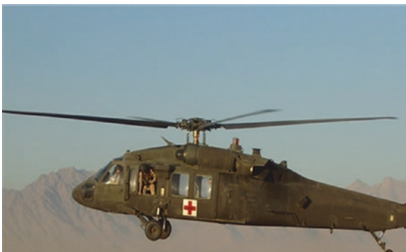
Fig. 41.2 MEDEVAC helicopter in Afghanistan. Casualty transport is most commonly by the Black Hawk helicopter. These helicopters can carry two litter patients and four non-litter patients depending on how they are configured. Certain configurations allow for four litter patients. The Black Hawk is the most common means for combat casualty transport from point of injury to the first role of care in the current battlefield system of care
