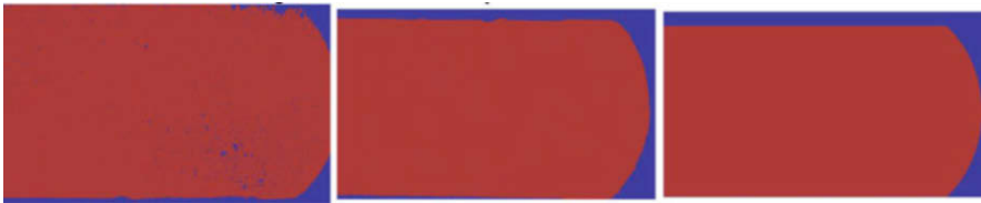
Fig. 18 The mask of the identified component in each of the resampled datasets: EBSD (left), BSE (middle), and DEFORM ® (right)
