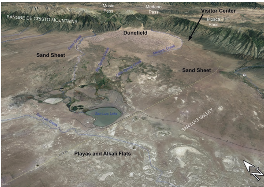
Fig. 7.1 Oblique view of Great Sand Dunes aeolian and hydrologic systems. Aeolian transport begins in the playas and alkali flats, where lunettes develop on the northeast side of the playas. Sand is transported across the sand sheet as indicated by parabolic dunes. Wind regime is altered by the mountain passes and sand accumulates as reversing and star dunes in the dunefield. Stream flow that originates in the passes flows around the dunefield, modifying the dunefield perimeter. Groundwater recharge occurs along the mountain front at a level the produces groundwater discharge areas downgradient producing gaining streams such as Big and Little Spring Creeks. Except during very wet periods, the playas are the terminus of the hydrologic system and water exits via evapotranspiration. Vertical exaggeration = 1.5
