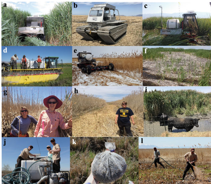
Fig. 13.6 Phragmites management: (a) Loglogic Softrak, marsh-capable equipment driving through a vast expanse of phragmites, (b) Marsh Master amphibious equipment used for phragmites herbicide and mowing management, (c) Loglogic Softrak being used for herbicide application to phragmites, (d) Wilco amphibious equipment used by the US Fish & Wildlife Service for phragmites management at the Bear River Migratory Bird Refuge (see Fig. 13.4), (e) Loglogic Softrak dragging a roller/crusher to break down phragmites litter in winter, (f) phragmites litter from winter mowing with live phragmites emerging in spring, (g) phragmites litter waist to shoulder high on wetland researchers Brittany Duncan and Karin Kettenring, (h) phragmites mowed to provide cattle access for grazing research study by Brittany Duncan, (i) cattle grazing phragmites-invaded wetland, (j) loading hydroseeding tank with native seeds, a tackifier, and mulch prior to seeding by David England, Emily Tarsa, and Keith Hambrecht, (k) seeds in paint strainer mesh for cold stratification prior to hydroseeding, and (l) hydroseeding by David England and Chad Cranney at Farmington Bay WMA
