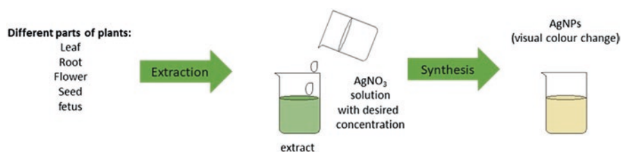
Fig. 7.2 Schematic representation of green synthesis of silver nanoparticles by plant extract
