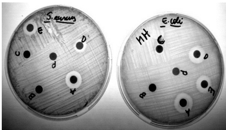
Fig. 8.7 Disk diffusion test. Legend: A—AgNO 3 , B—Extract of Melissa Officinalis leaves, C—AgNP1 (0.05 mg/L), D—AgNP2 (0.5 mg/L), E—AgNP3 (1.2 mg/L), P—phosphate buffer saline (PBS)
