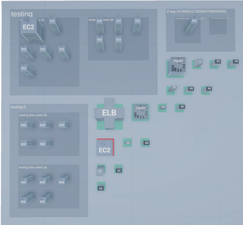
Fig. 9. An example of the rectangle packing layout for a considerable size infrastructure, composed of: three Auto Scaling Groups containing multiple size instances and two Scaling Policies; a stopped Virtual Machine; one Load Balancer and several Security Groups [32].
