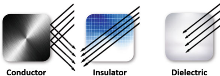
Fig. 2.1 Interaction of microwave with conductor, insulator, and dielectric materials
