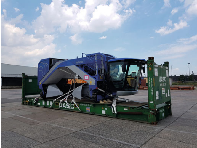
Fig. 14.2 OOG example: Harvester machine on flat rack
