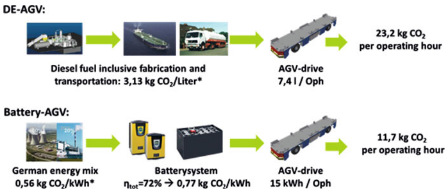
Fig. 5.8 AGV well-to-wheel GHG production for Diesel-Electric (DE) and battery drivetrain
