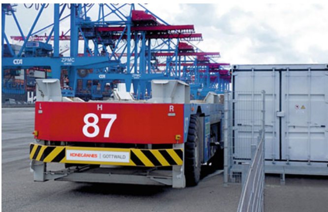
Fig. 5.12 Li-Ion battery-AGV at an AQC at CTA, Hamburg
