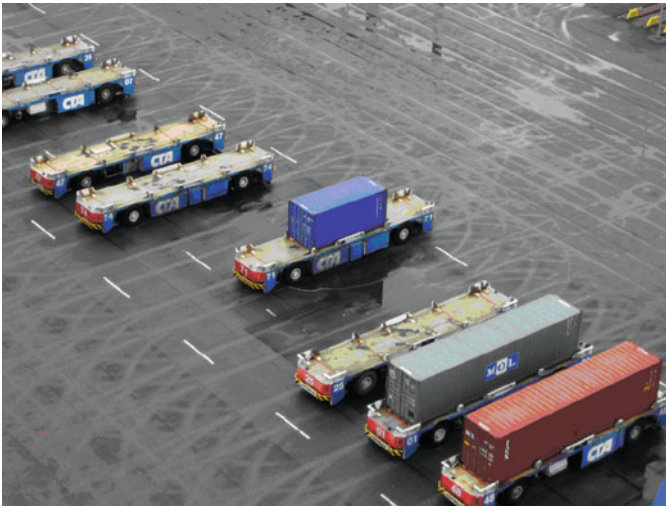
Fig. 14.7 AGVs in the waiting/holding area at the CTA in Hamburg
