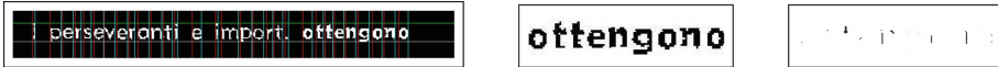
Fig. 6. Word segmentation (left) and identification of bold words: on the center we show one bold word and the results of the erosion on the right.
