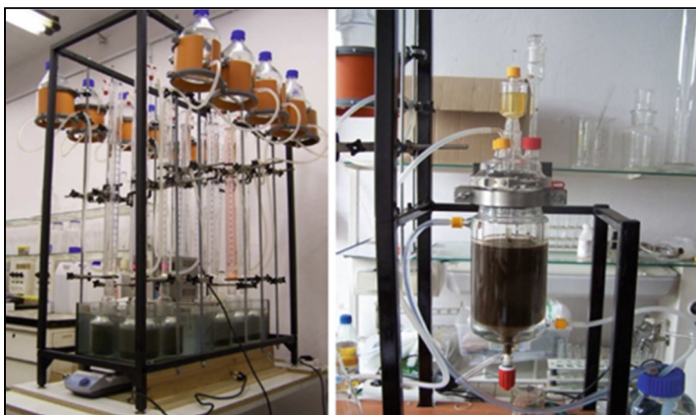
Fig. 2. Research stand for the study of biogas productivity of substrates according to DIN 38414 S.8 (left), inoculum station for quasi continuous fermentation work (right) (own source)
