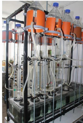
Fig. 2. Research station scheme for methane fermentation process: 1. water heater with temperature regulator, 2. glass water jacket, 3. reactors with a capacity of 1 \text{ dm}^3 , 4. cylindrical tanks in which gas is stored with a capacity of 1.2 \text{ dm}^3 , 5. shut-off valve, 6. gas flow meter, 7. equalizing tank, 8. measuring station: gas analyzer AG-BIO by Alter, pH-meter, CP-215 by Elmetron, two temperature sensors, multimeter CX 401 by Elmetron
