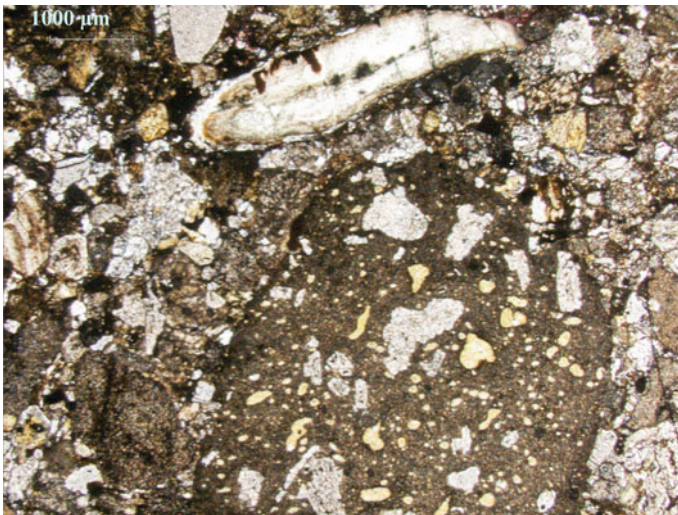
Fig. 1 Photomicrograph in plane polarized light showing the matrix in conglomerate of Smith Island, North Andaman with clasts of various composition viz., shale, mudstone, ophiolites, trachy andesite
