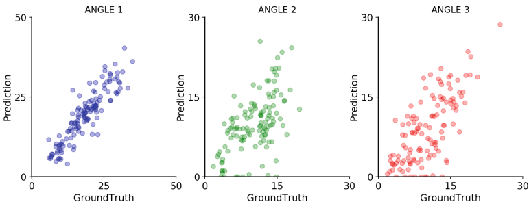
Fig. 4. The correlation coefficients between three angles predicted by the proposed method and ground truth. The angles are numbered from top to bottom and our method has much better performance on the first angle.
