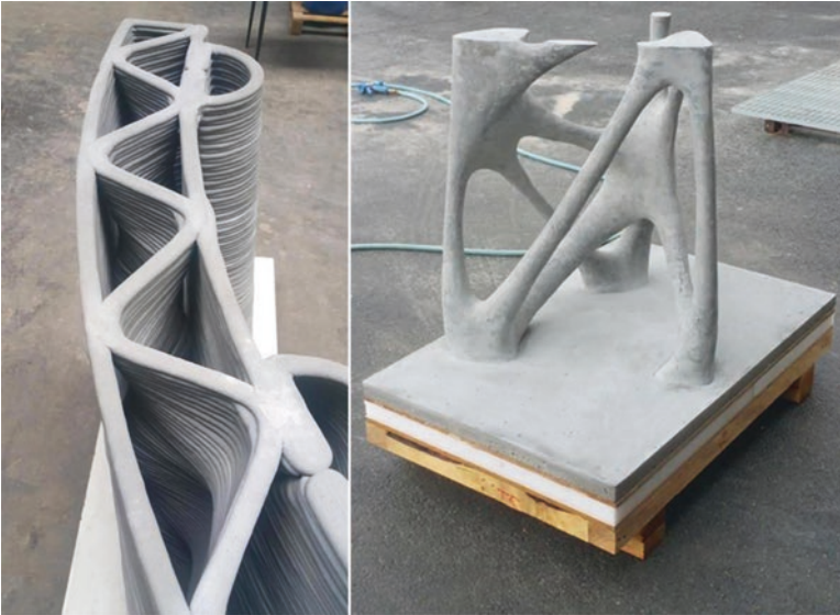
Fig. 16 3D-printed UHPC curved wall (left) and free-form structure (right) (XTreeE and LafargeHolcim)
