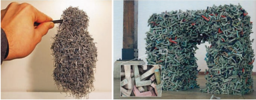
Fig. 15 Entangled assemblages of non-convex particles which could provide self-assembled reinforcement for concrete. Left: an aggregate of staples. Pick one; take them all. Right: a self-standing structure of Z-shaped particles (Kieran Murphy, Leah Roth, Heinrich Jaeger, Project Z-Form)
