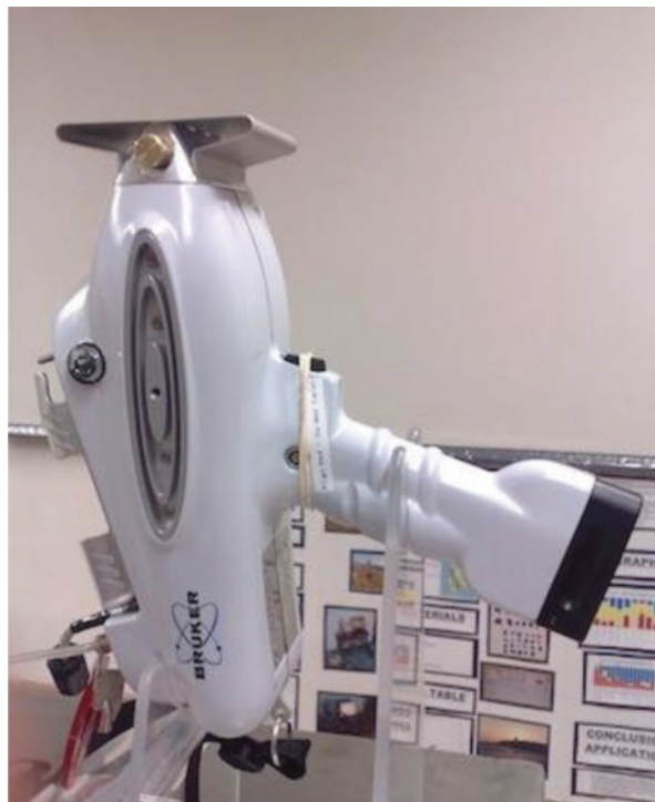
Fig. 5 pXRF at the Archaeological Science Laboratory, University of South Florida, Tampa. The lightweight of pXRF (2 kg/4.49 lb) allows users to conduct the analysis in the laboratory or in situ. (Photo by Hasan Ashkanani)
