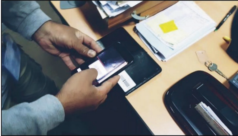
Fig. 12 Showing a technician accessing Bar Cloud System through a portable device and using assets barcode scanning feature
