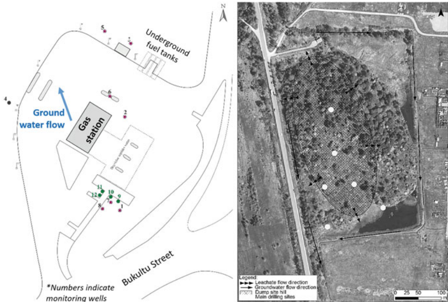
Fig. 3 Gas station monitoring and air sparging (thermal treatment) well-planning scheme in Riga gas station (left); Kleisti dump site before remediation—large dots drilling sites in waste mass, small dots monitoring wells for remediation planning (right)
