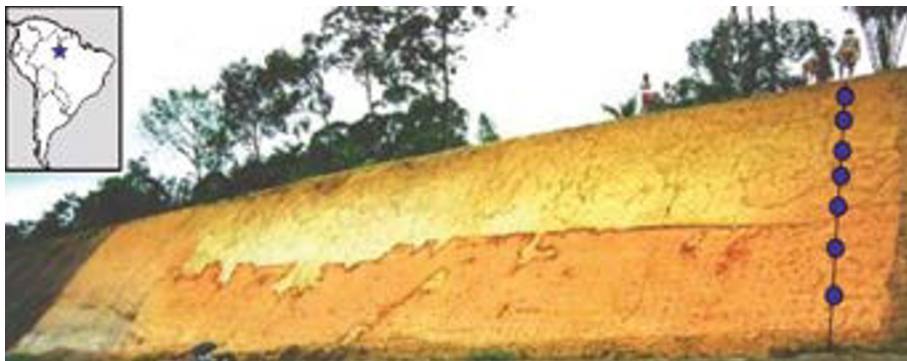
Figure 5.6 - Vertical section showing the different horizons of a lateritic soil from the Manaus region. Samples were collected at the seven levels indicated by the circles. The structures observed on the section (discolouration, indurated iron-oxide-rich line) reflect recent re-mobilisation of iron due to fluctuations in the reduction-oxidation conditions which did not affect the kaolinites.
