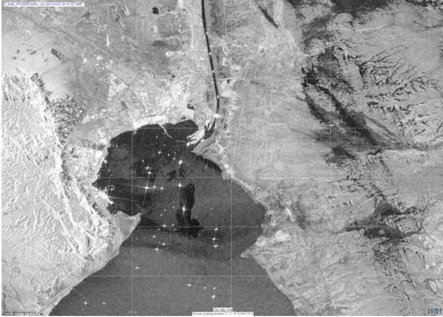
Fig. 12.11 SAR Sentinel-1A image of Suez Port on 01 April 2019, 03:45:02 GMT. Black patches are oil spills, and white dots are ships
