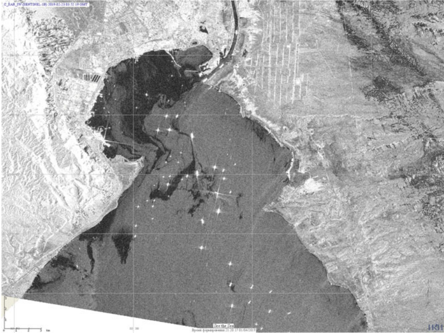
Fig. 12.9 SAR Sentinel-1B image of Suez Port on 23 February 2019, 03:52:19 GMT. Black patches are oil spills, and white dots are ships
