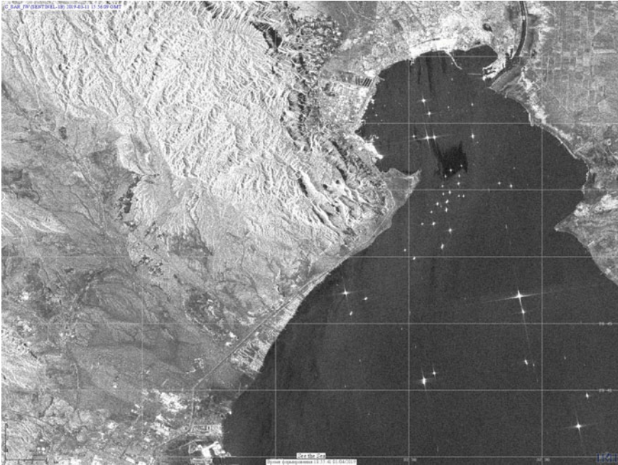
Fig. 12.10 SAR Sentinel-1B image of Suez Port on 11 March 2019, 15:56:09 GMT. Black patches are oil spills, and white dots are ships
