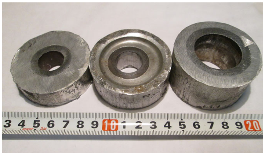
Fig. 4 Bimetallic samples obtained by joint stamping of liquid aluminum AK9ch and sintered powder ANS100.29
