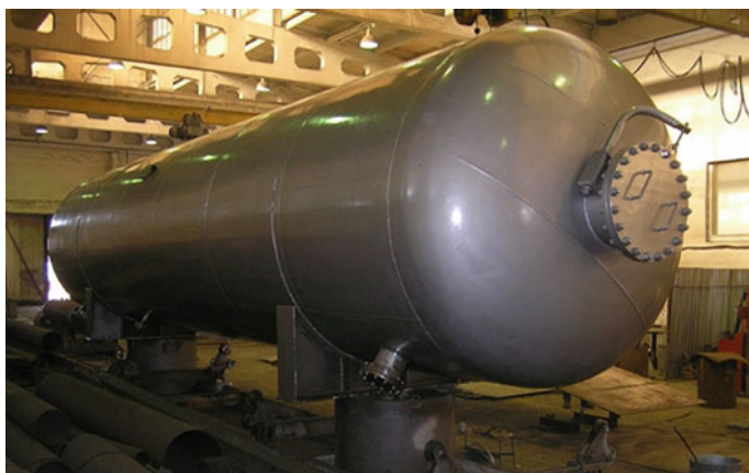
Fig. 1 Welded vessel for transportation and storage of cryogenic liquids
