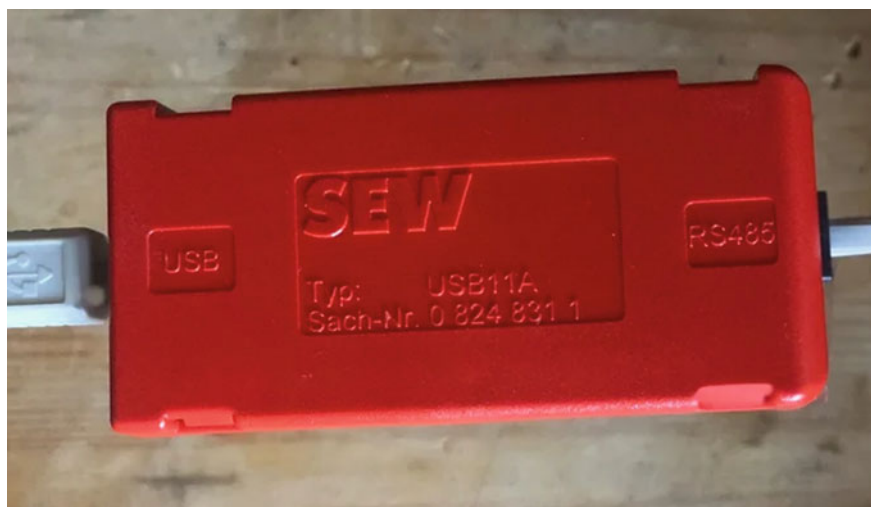
Fig. 2 SEW-EURODRIVE converter for PC connection to RS485
