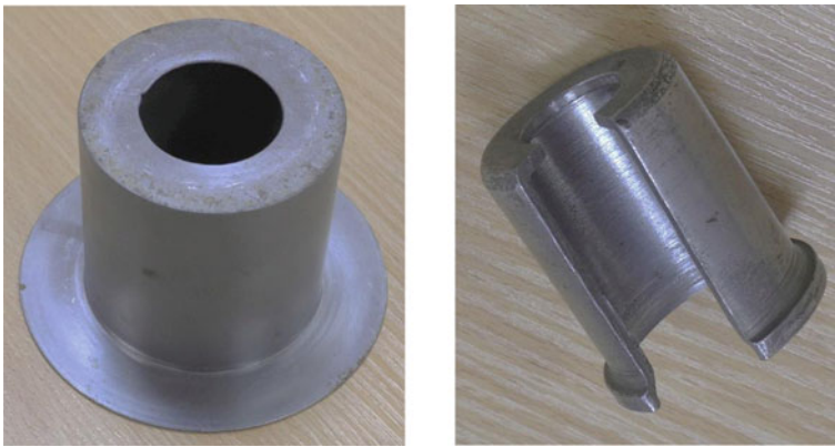
Fig. 8 Inner flanges rotary forged from thin-walled tubes
