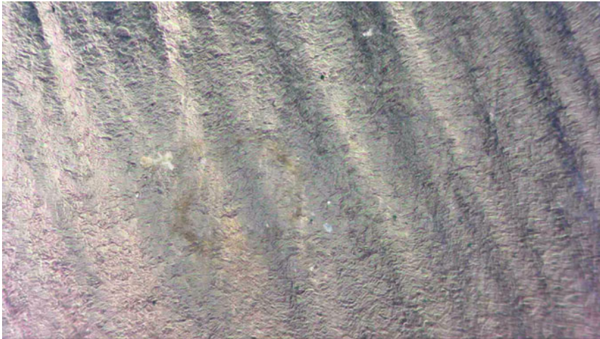
Fig. 4 The surface after electrolyte-plasma polishing of steel 15KhNFSH, magnification \times 250
