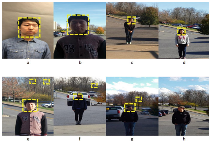
Fig. 3 Successful cases of face detection via the Viola Jones algorithm on cell phone images are shown in “a–d”, while “e–g” represent cases with false positives, in which a non-face region has been falsely identified as a face, and “h” demonstrates false negative, in which a face was falsely not identified
